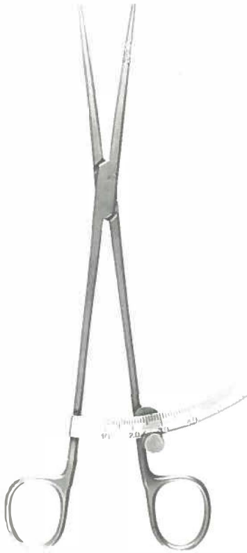
Figure VI.2: A pair of compasses with an externally readable scale, constructed for measuring of the frozen area on the portio (The width of the compasses can be fixed with a screw).
