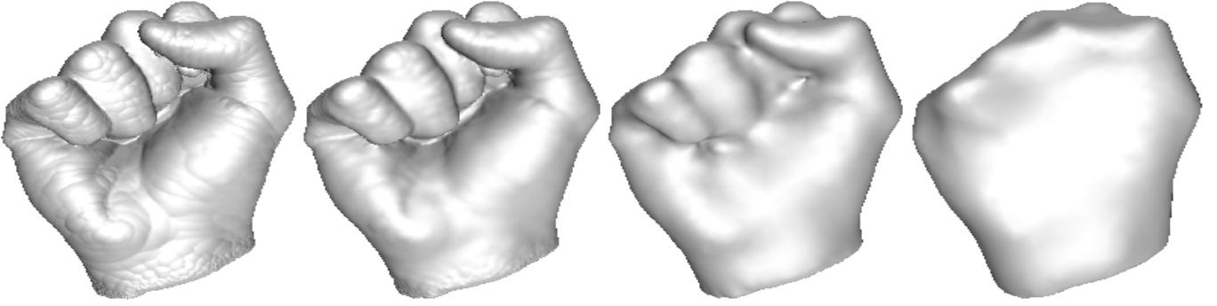
Figure 2: The approximating skin surface of a set of balls forming a hand. The patches between the maximal balls become larger as the shrink factor is decreased. The shrink factors (from left to right) are 0.95, 0.8, 0.5 and 0.2.
