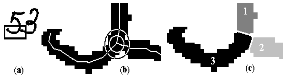
Figure 3: Orthogonal cuts: (a) Original image (b) Potencial region (c) Cuts realized
