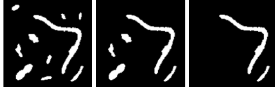
Figure 2. Binary attribute filters applied to an image of bacteria: (left) original; (middle) area opening using area threshold \lambda = 150 ; (right) elongation thinning using attribute I/A^2 > 0.5 .
