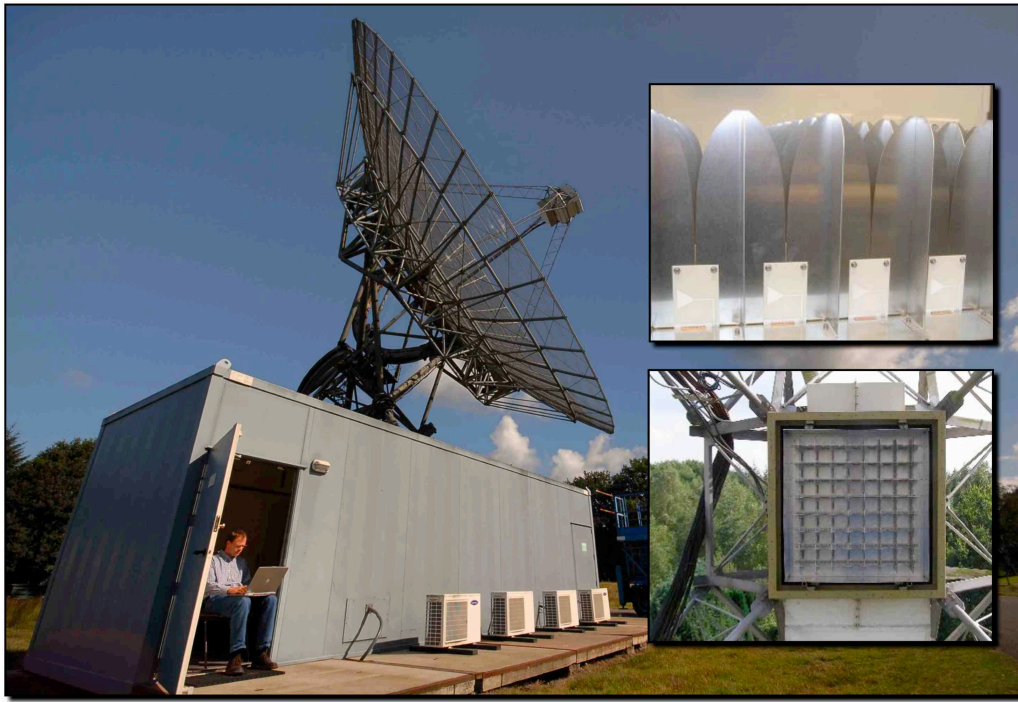
Figure 2. The WSRT telescope RT5 equipped with the APERTIF prototype. Shown in the inserts is the Vivaldi array in the lab (top right) and in the focal plane of the telescope (bottom right).
