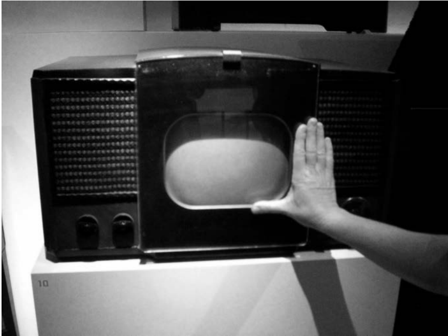
Fig 1: RCA's 1946 630-TS television set with a screen size of only 10 inches diagonally.
