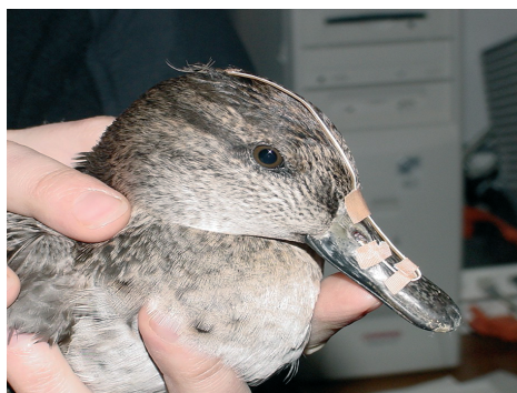
Teal ( Anas crecca ), equipped with a thermistor for the measurement of T_{exh} (chapter 5).
