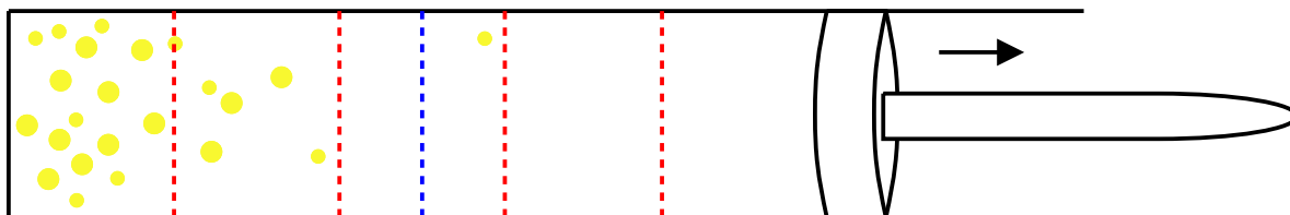
Figure 4.4: Abstract Piston with Representative Partitions: Blue Line for 2 Bins, Red Line for 5 Bins.
