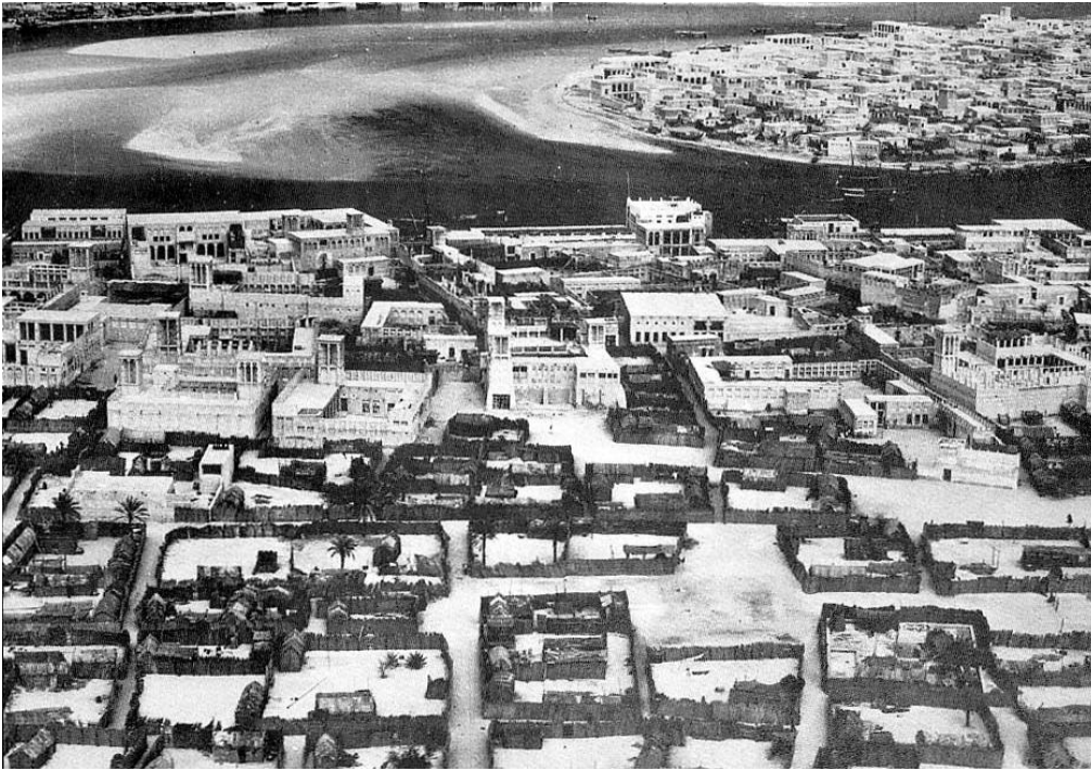
Figure A: The urban fabric and density in the 1950s. Houses were built intentionally in clusters to achieve privacy and collective tribal safety. The clusters were linked by narrow pathways designed for pedestrians, as well as for animals that were used to carry goods and water (Sunders, 2003)
