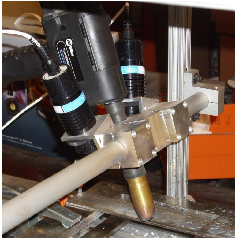
Figure A-10: IR pyrometers mounted to the welding test station (Ely, 2010)
