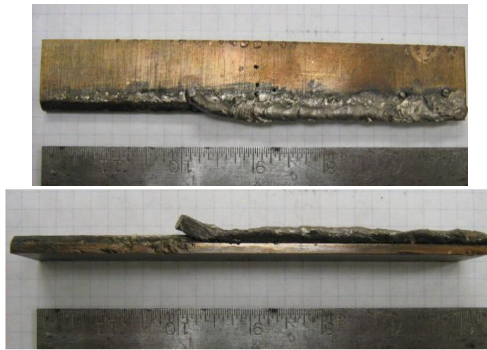
Figure 2-6: Trial 7 from top and side views after attempting to delaminate filler metal
