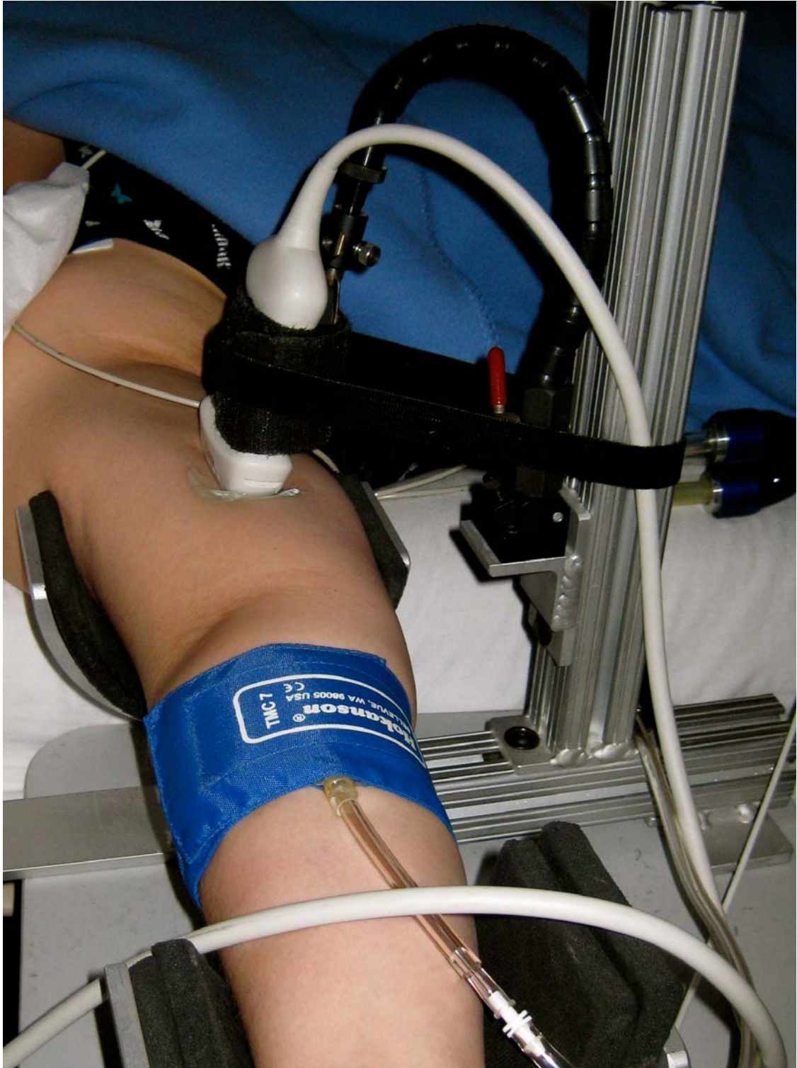
Image 2C. Arm support system used for FMD data collection.
