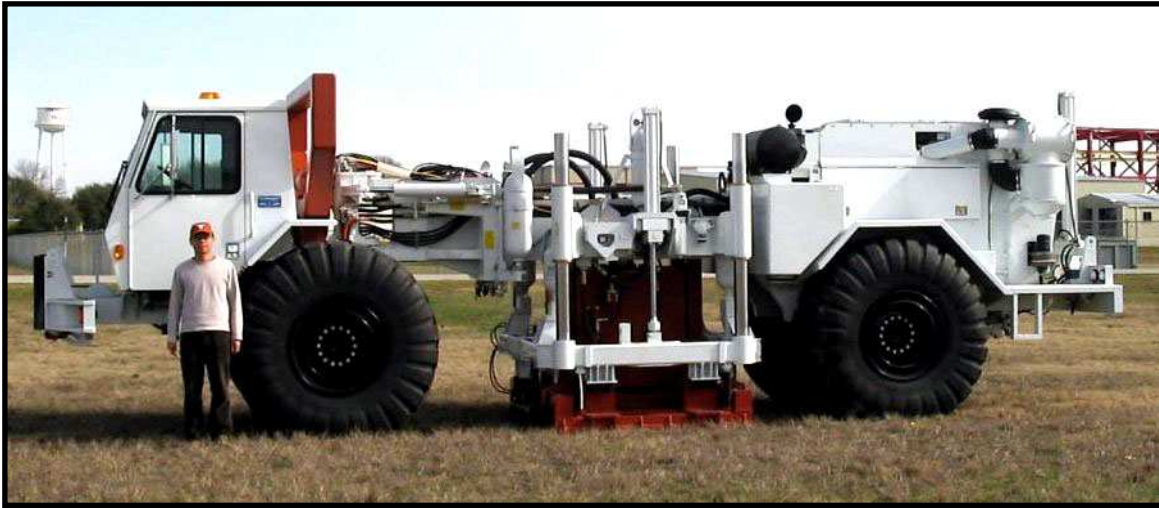
Figure 5.3 Liquidator Used as a Seismic Source at the Hornsby Bend Site (Courtesy of NEES@UTexas)
