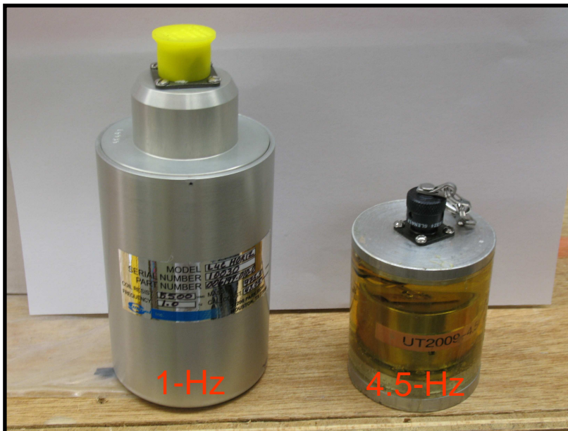
Figure 5.7 1-Hz and 4.5 Hz Geophones used at the Hornsby Bend Testing Site
