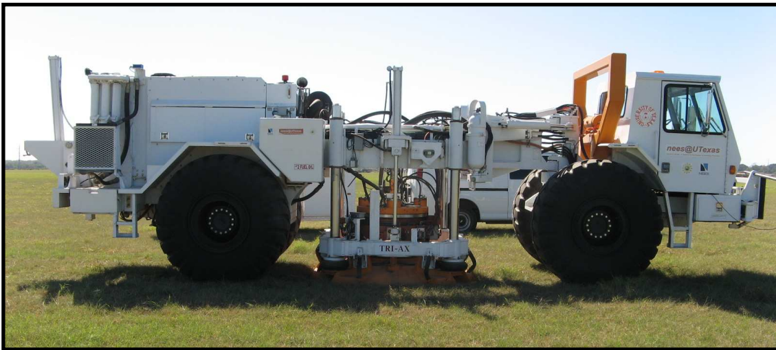
Figure 5.4 T-Rex Used as a Seismic Source at the Hornsby Bend Site (Courtesy of NEES@UTexas)
