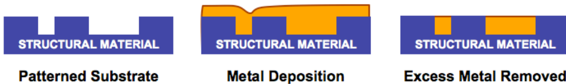
Figure 2.9: Illustration of the damascene process in which a substrate is patterned, coated with a noble metal, and excess metal is polished off.
