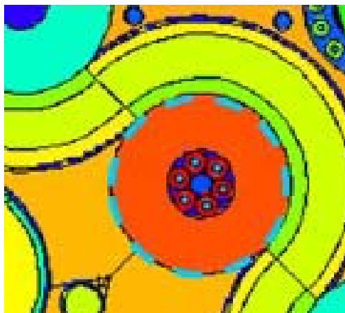
Figure 10, the surface source substitution method developed by Wilson and Schneider. Note the dash-lined circle as the surface source.
