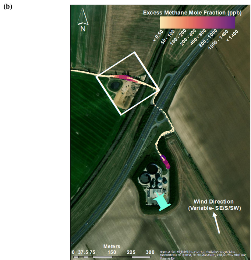
Fig. 1. a) Downwind plumes of biogas plant A sampled during a 1-hour period of a mobile survey on 30 January 2020. (b) ArcGIS map of excess CH 4 mole fraction above background in ppb, as a top view of downwind plumes of plant A. White arrows show the wind direction. White box represents the data used in emission rate calculation. Green pin indicates the site of biogas plant A. The surveyed road was reached after passing under the highway. (For interpretation of the references to colour in this figure legend, the reader is referred to the web version of this article.)
