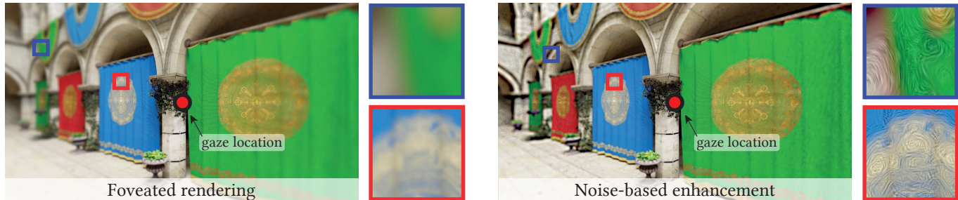
Fig. 1. Our method enhances the output of standard foveated rendering (left) by adding carefully tuned procedural noise (right). The enhancement replaces accurate rendering of spatial details, which are detectable but not resolvable by the human visual system, and allows applying more aggressive foveation during the rendering process. This images are designed to be viewed at an 80-degree wide field-of-view, with gaze at the center. Scene courtesy of Morgan McGuire and Frank Meinl, Crytek.
