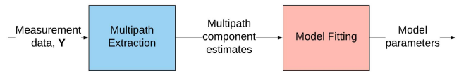
Fig. 1. Calibration procedure usually followed where estimates of multipath components are used as summaries.
