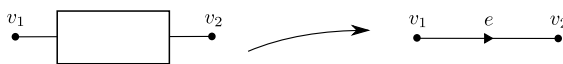
Fig. 7. Deriving the underlying graph of a capacitance, conductance, ideal diode, PN-junction diode, inductance, resistance, or sources.
