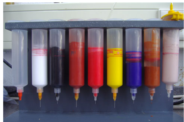
Fig. 2 Syringes filled with pigment pastes (Factor 2; Flagstaff, USA) connected to air pressure with a yellow coloured adapter
