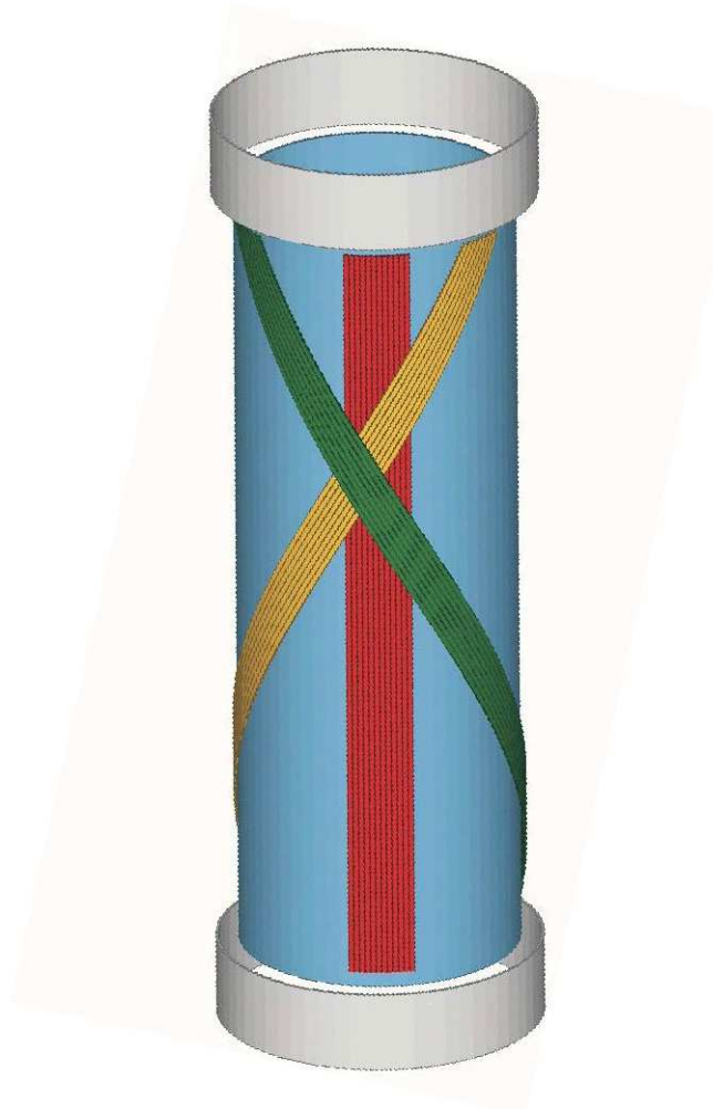
Figure 7: Arrangement of scintillator strips mounted on the detector. PMTs and front-end electronics are mounted in the ringed regions on each end of the detector. [1]
