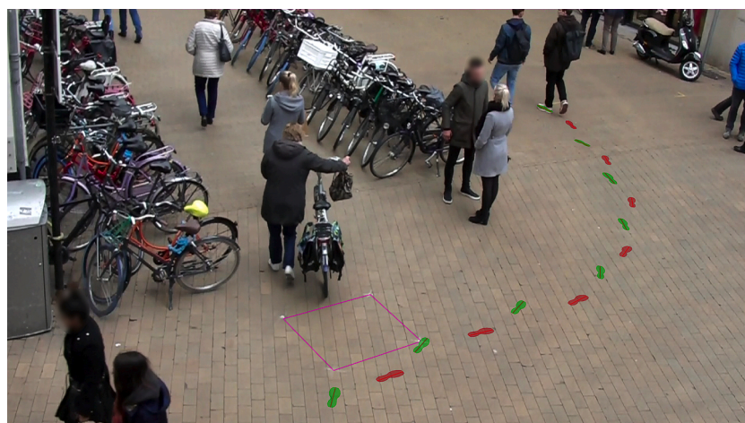
Fig. 1. Image plane of the MovieProcessing package. The marked footprints show the walked trajectory of participant four. The purple square shows the perspective correction. The red footprints correspond to the right foot and the green footprints to the left foot (For interpretation of the references to colour in this figure legend, the reader is referred to the web version of this article).
