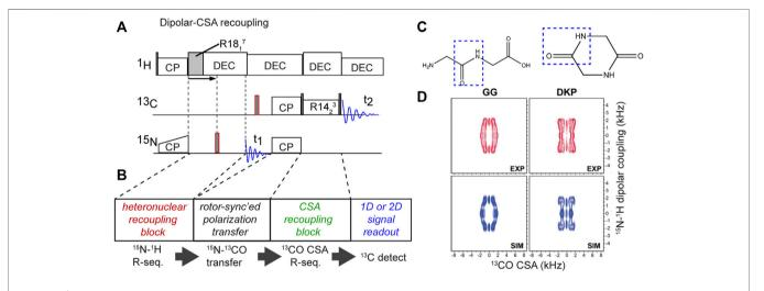
**FIGURE 9** | Hybrid CSA/dipolar recoupling experiment. **(A)** Pulse sequence and **(B)** its building blocks. **(C)** Chemical structures of test molecules with different molecular configurations mimicking the cis or trans peptide bond angle  $\omega$ . **(D)** 2D CSA-dipolar correlation spectra for the two reference compounds representing the distinct  $\omega$  angles. Panel (D) was adapted with permission from ref. (Mukhopadhyay et al., 2018).
