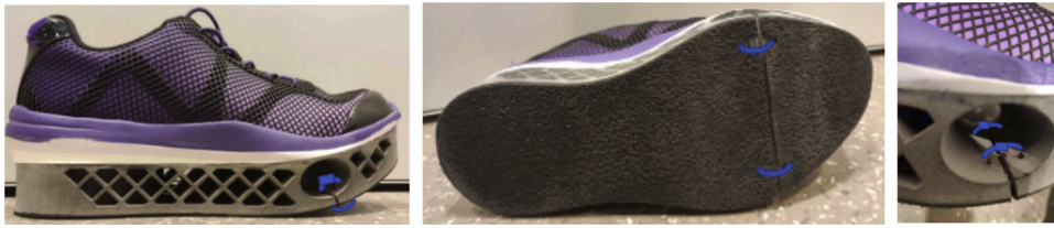
Fig. 2. Experimental shoe with a forefoot rocker radius of 210 mm. Cable ties were used to increase LBS of the rocker sole (graphically visualized in blue). Cable ties were fitted in the holes and did not stick out the bottom nor effect sole geometry. Shoe soles had a thickness of 35 mm and toe spring of 20 mm.
