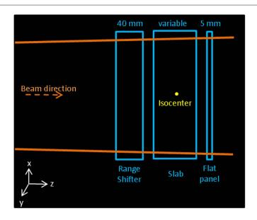
**Figure 1.** Schematic representation of the simulated elements for FP-PR calibration. The edges of the PR field and the beam direction are depicted in orange. The isocenter is shown in yellow. Three water blocks on the beam path were simulated along the z-axis to represent a range shifter, a water equivalent slab of varying thickness and the FP detector. The thickness of each water block is indicated in the schematic.
