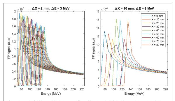
**Figure 2.** Two calibration datasets, with  $\Delta X=2\,$  mm and  $\Delta E=3\,$  MeV (left) and with  $\Delta X=10\,$  mm and  $\Delta E=9\,$  MeV (right). ERDFs are represented in different colors, corresponding to thicknesses from 0 to 80 mm. For each plot, the left-most ERDF corresponds to  $X=0\,$  mm and the right-most ERDF corresponds to  $X=0\,$  mm. The legend in the left side plot is omitted for readability.
