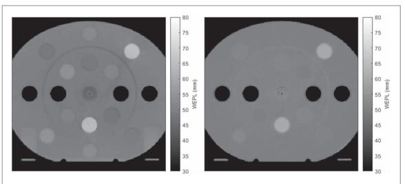
**Figure 3.** WEPL images in mm resulting from FP-PR simulations using a calibration with  $\Delta X=2$  mm and  $\Delta E=3$  MeV (left) and  $\Delta X=10$  mm and  $\Delta E=9$  MeV (right).
