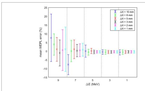
**Figure 4.** Mean and standard deviation (error bars) of the WEPL relative error (%) for all calibration settings. Different  $\Delta E$  values are shown across the x-axis, and different marker colors stand for different  $\Delta X$  values.
