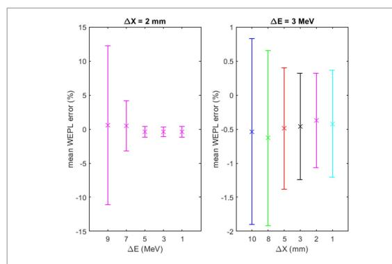
**Figure 5.** Mean and standard deviation (error bars) of the WEPL relative error (%), as a function of different  $\Delta E$  values using a fixed  $\Delta X = 2$  mm (left side graph), and different  $\Delta X$  values with a fixed  $\Delta E = 3$  MeV (right side graph).
