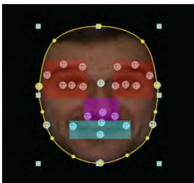
Figure 2. Face tracking in Adobe After Effects CC. The yellow line is the ellipsoid mask after automatic alignment to the contours of the face. Each circled cross is a face track point. The colored rectangles indicate the locations of the different areas of interest (AOIs); the red rectangles denote the right- and left-eye AOIs, the purple rectangle shows the nose AOI, and the blue rectangle specifies the mouth AOI.
