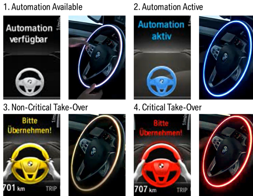
Fig. 3. The visual interface modalities in the speedometer and the illuminated steering wheel.
