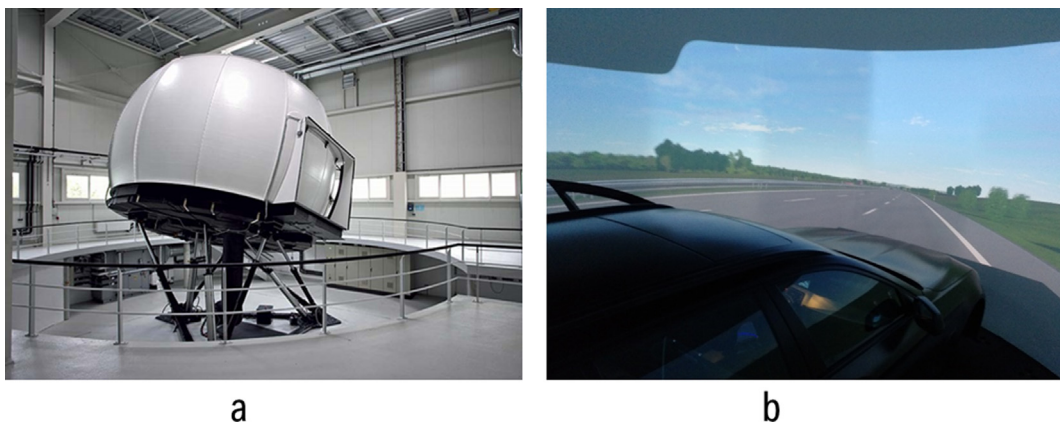
Fig. 1. Exterior view of the dynamic simulator (a) and interior view (b).
