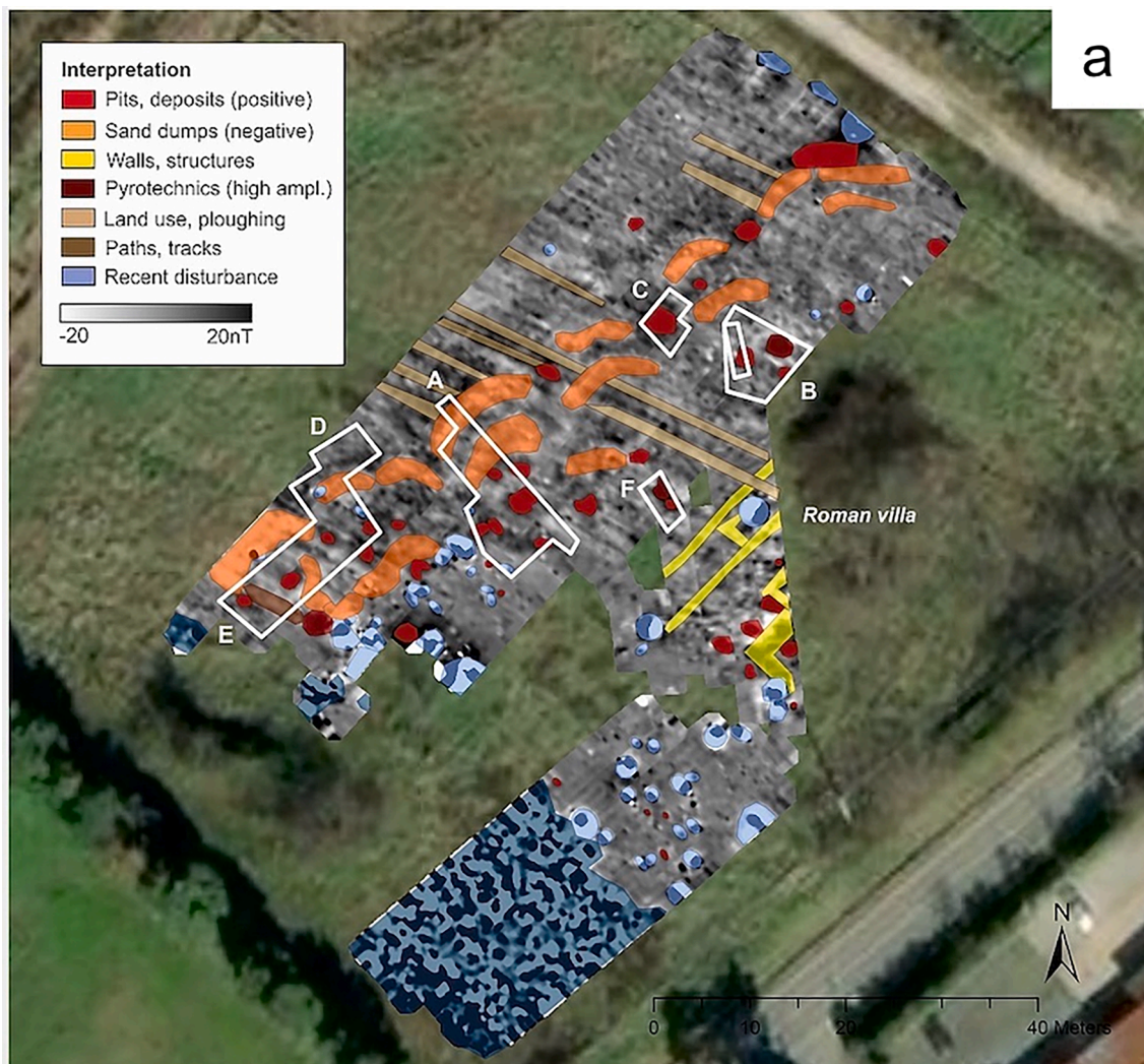
Fig. 2. a) Geophysical survey (above) with interpretation of features. Excavated areas are indicated by capital letters; b) Features studied and excavation areas: 1 = dump of fragments of briquetage vessels; 2 = infilled pits in excavated area B; 3 = geomagnetic map of excavated areas B and C with the infilled pit studied (feature B1).
