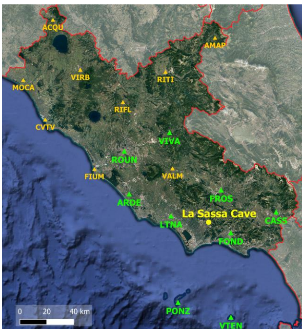
Figure 2 – The permanent GNSS stations of the Lazio Region: in green the stations used in the computation of the VRS.
