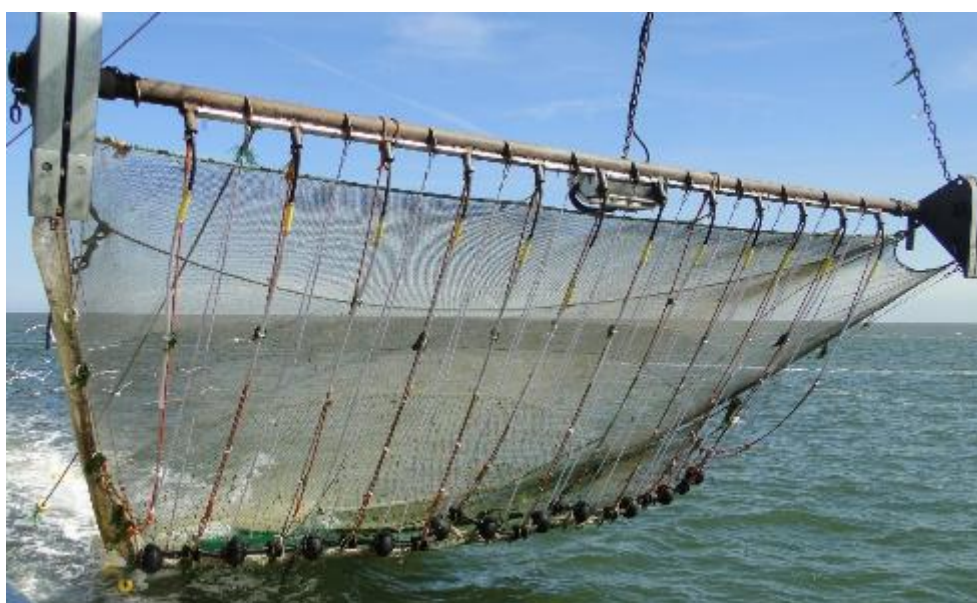
Fig. 2-6 - Image of a pulse trawl design that is being used today on the Dutch Wadden Sea by HA 31. The gear is characterised by the use of a straight, lightweight bobbin rope with 11 ellipsoidal bobbins (instead of 36 bobbins in the previous traditional
