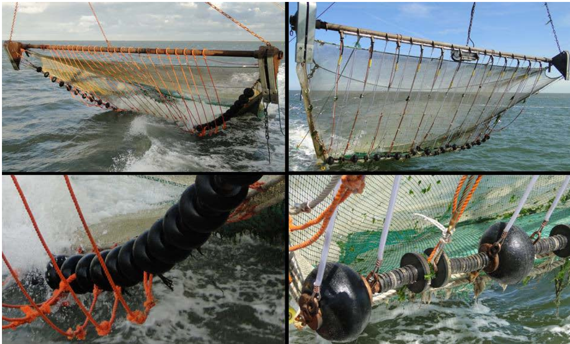
Figure 5.1: Front view (top) and details of the bobbin rope (bottom) of a traditional trawl with 36 bobbins in a u-shaped bobbin rope (400 kg, left) and a pulse trawl with 11 bobbins in a straight configuration (150 kg inclusive of electrodes, right) illustrating the difference in mechanical stimulation and the size and orientation of escape opportunities between the bobbins for by-catch species
