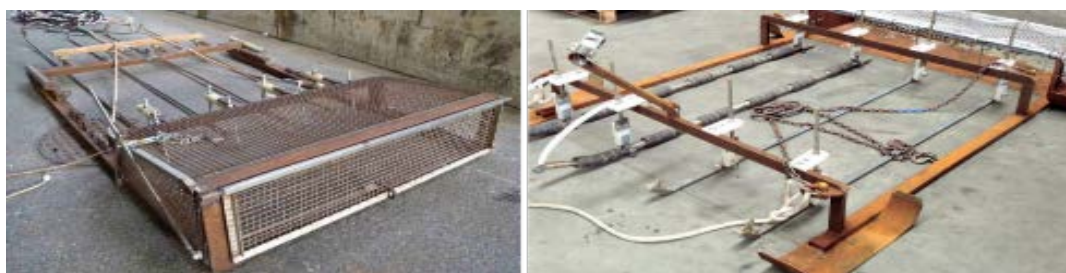
Fig. 2-10 - Two different prototypes of pulse dredges that were developed and tested in Irish (left) and Dutch (right) razor clam fisheries. Right picture modified from Breen et al. (2011) and left picture from Visserijnieuws (2015).
