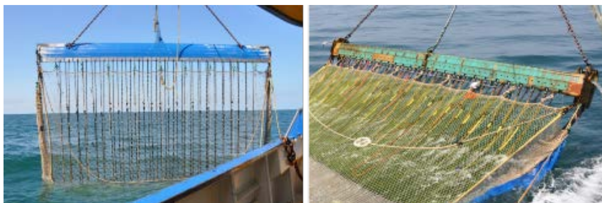
Fig. 2-9 - Pulse SumWing by HFK Engineering (left) and Delmeco Multiwing (right). Both gears are used today in the Dutch flatfish pulse fishery. Around 90 vessels are equipped by either Delmeco or HFK according to a ratio of approximately 1 to 5 respectively.
