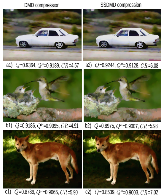
Figure 4: Comparison of DMD (a1–c1) with SSDMD (a2–c2) for three focus-and-context images. For each image, we show the standard MS-SSIM quality Q , spatial-saliency-aware MS-SSIM Q^\mu , and compression ratio CR.
