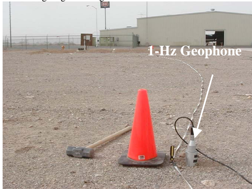
Figure 2.15 Photograph of 1-Hz Geophone on the Yard of the Brawley Airport in Imperial Valley, CA
