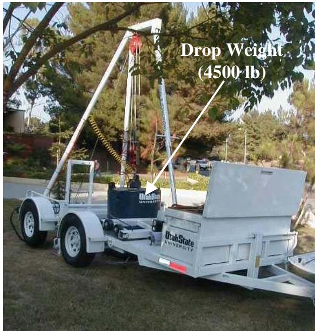
Figure 2.10 Large Drop Weight Used as Impact Source to Perform SASW Test at LA Fire Station #99, Los Angeles, CA
