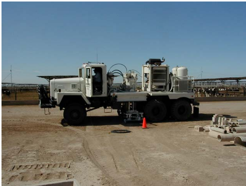
Figure 2.11 A Traditional Vibroseis Performing the SASW Test at El Centro Array #1 in Imperial Valley, CA
