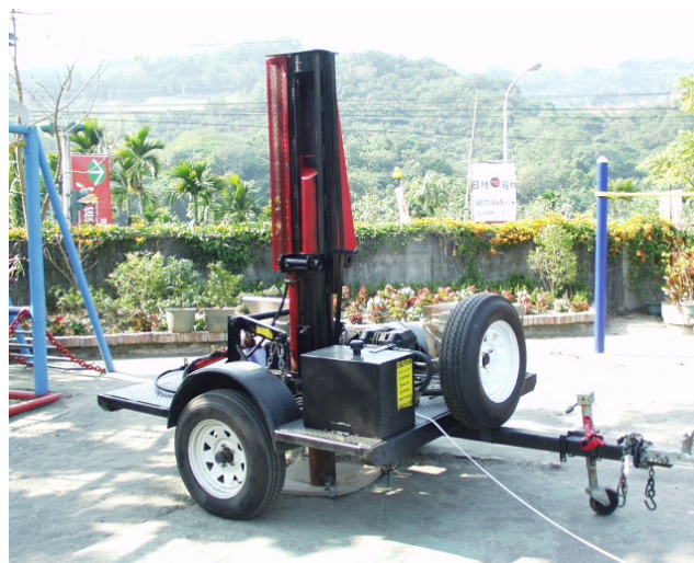
Figure 2.9 DynaSource Used as Impact Source at Kung-Chung Elementary School Site (TCU-52) in Taiwan
