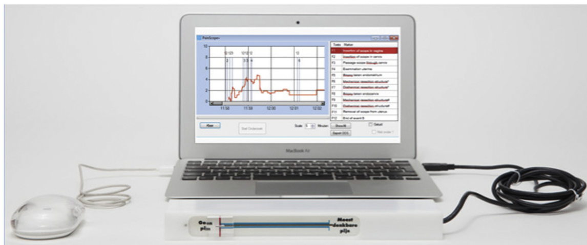
Fig. 1. The Continuous Pain Score Meter: laptop with the software (PainScope) and the pain slider.
