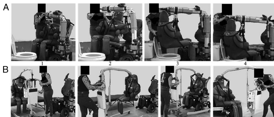
FIGURE 2. A participant performing a transfer with the Hoyer Advance (A) and SA (B) at two different transfer surfaces. 1, lift phase; 2–3, transport phase; 4, placement phase.
