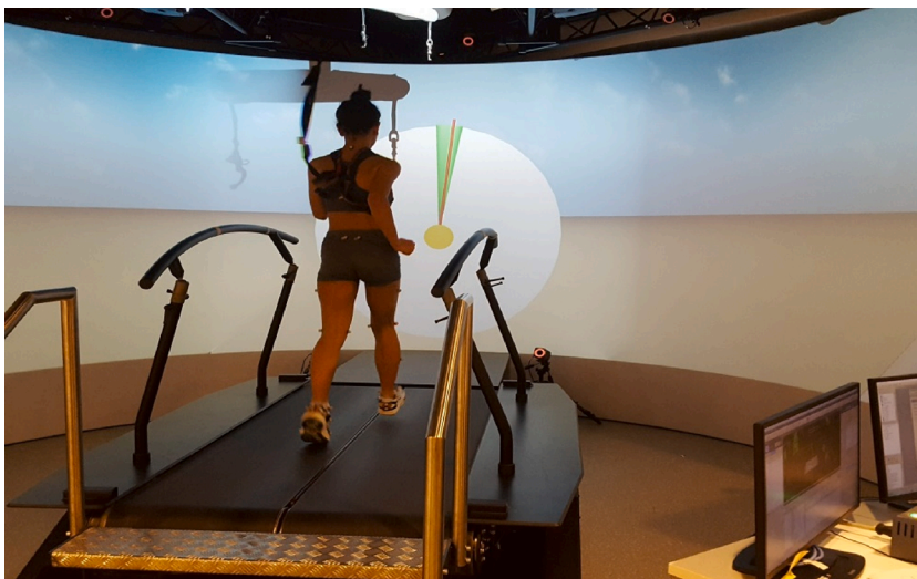
Fig. 2. Picture representing real-time visual feedback for changing FPA. The training process: real-time visual feedback is provided to the subject via the big screen. The red pointer represents the FPA of the right foot that is fixed in midstance (50 % stance phase) and updated at each step. The target area is a wedge with a 5° range, with its middle point specifying the subject's normal FPA. The aim is to turn the target area green (positive feedback) by keeping the red pointer (FPA) inside the target area. If the red pointer leaves the target area, the target area turns red (negative feedback). (For interpretation of the references to colour in the Figure, the reader is referred to the web version of this article).
