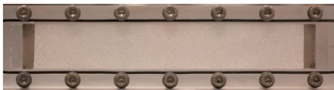
Fig. 2. Device used for flow cell experiments with glass beads (top view).
