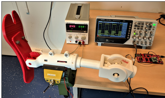
Fig. 4. Test setup used for testing the algorithms on the Prosthesis showing the PIC32 micro-controller, power supply and the scope.
