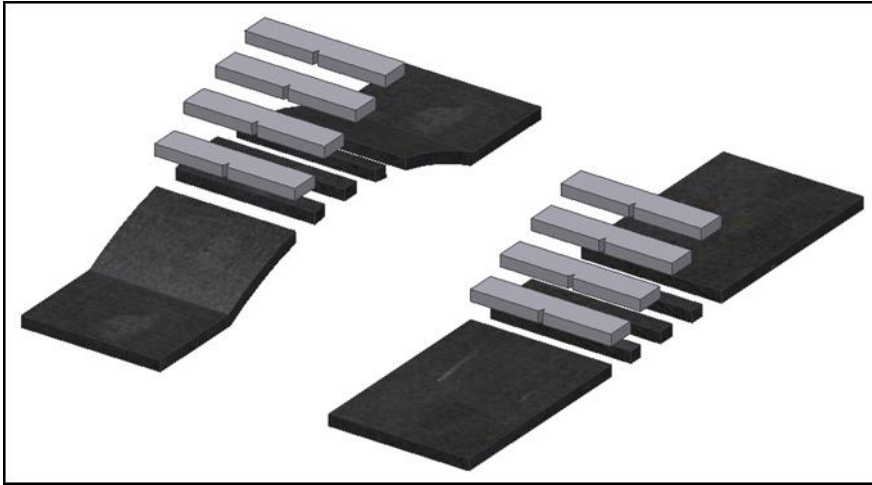
Fig. 4.4: Positions of Charpy V-notch samples.
