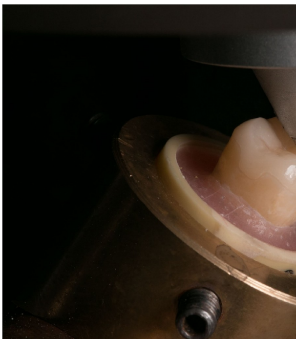
Fig. 2. Sample in universal testing machine at 45° for load to fracture test. Force applied
