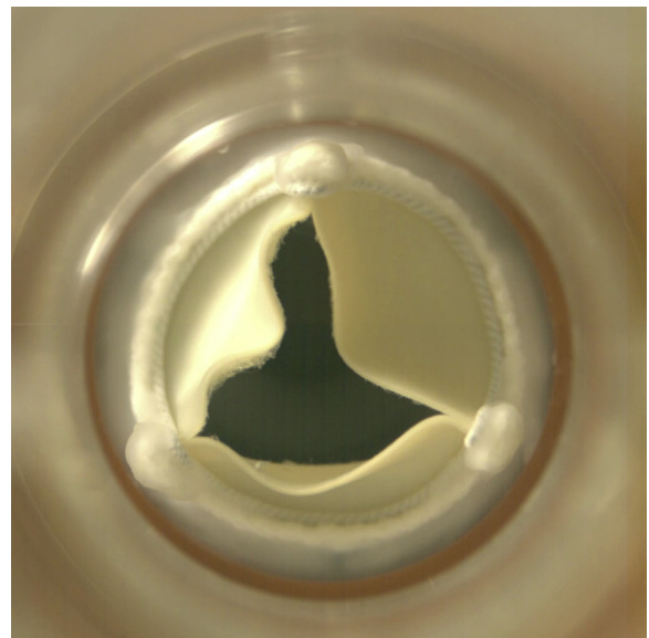
VIDEO 2. Opening and closing of a 25 mm Carpentier Edwards Magna Ease valve (Edwards Lifesciences, Irvine, Calif) under normal aortic pressure condition (120/80 mm Hg). Video available at: https://www.jtcvs.org/article/S0022-5223(19)31338-8/fulltext .
