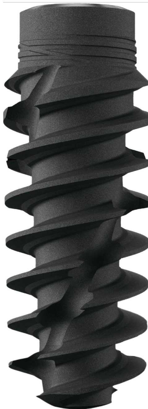
FIGURE 3: Straumann BLX implant RB. Roxolid® implant material with SLActive® surface. Full tapered core with self-cutting threads, chip flute for redistribution of bone chips, and microthreads on the implant neck to reduce stress at the cortical bone. Conical implant abutment connection (TorcFit™). Courtesy of Straumann AG.
