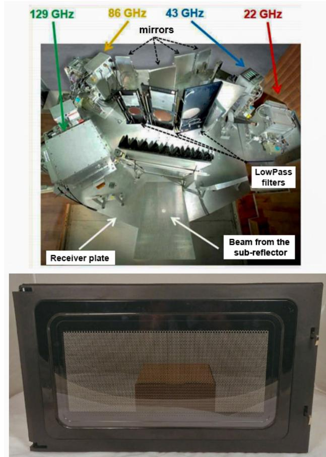
FIGURE 3.2: Applications of dichroic filters
