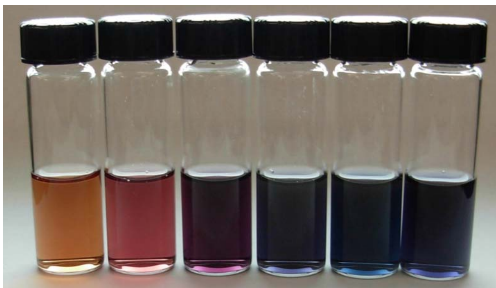
Figure 6.7: Color and clarity of each system studied at a molar ratio of (40:1) AA:Au, viewed in transmitted light. The vial on the far left is (7:1) Au:BSA from Chapter 3, produced by reduction with sodium borohydride, included for comparison. From left to right, the remaining vials contain (6:1) Au:BSA, (12:1) Au:BSA, (24:1) Au:BSA, (48:1) Au:BSA, and (96:1) Au:BSA.
