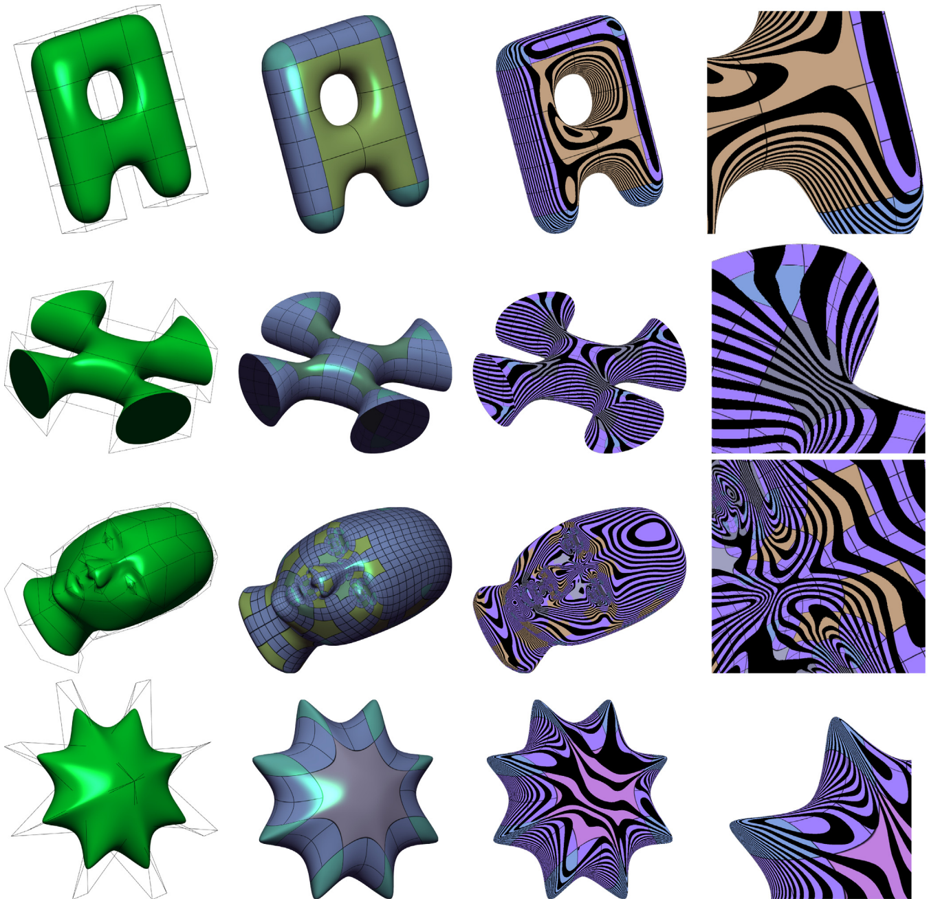
Fig. 6. Left: Shading and control mesh. Middle left: Shading with patch boundaries. Middle right: Reflection lines and patch boundaries. Right: Details of reflection lines and patch boundaries. Top to bottom: 12 triangles, 64 quadrilaterals, 12 pentagons; 8 triangles, 248 quadrilaterals, 8 hexagons; 84 triangles, 1656 quadrilaterals, 42 pentagons, 18 hexagons, 2 heptagons; 16 triangles, 64 quadrilaterals, 2 octagons.
