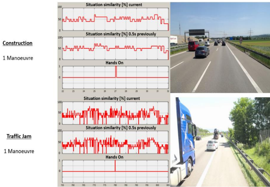
Figure 11. Two exemplary self-initiated take-over situations that were not trained in the training set. Predicted sideswipe manoeuvres never reach a confidence greater 80%.
