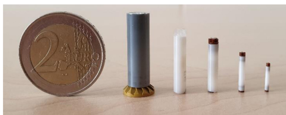
Fig. 1. Solid-state NMR sample sizes. Comparison (left to right) between the size of a 7 mm rotor spinning up to 7 kHz, a 4 mm rotor spinning up to 18 kHz, a 3.2 mm rotor spinning up to 24 kHz, a 1.9 mm rotor spinning up to 42 kHz and a 1.3 mm rotor spinning up to 70 kHz, including their driving caps, and that of a 2€ coin (far left).
