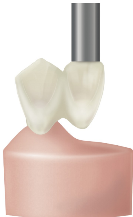
Fig. 3. Figure how the loadcell was applied on the incisal edge of the pontic.
