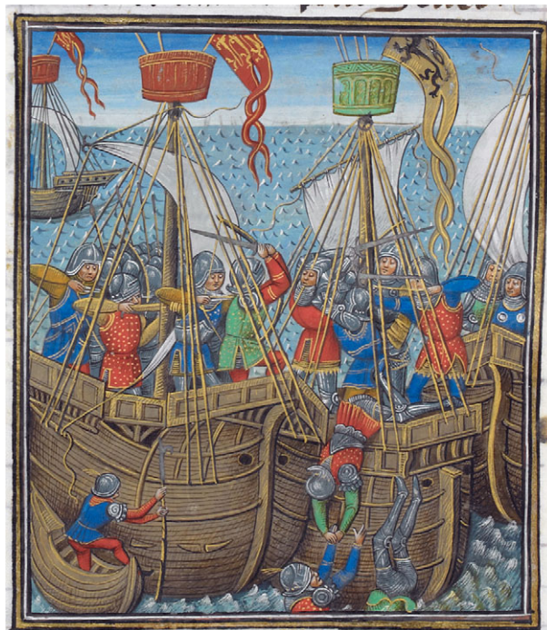
Figure 24. Late 15th-century illustration of vessels showing boarding and close combat. Note the wales and vertical reinforcements on the outside of the vessels (from Jean de Wavrin's Chronique d'Angleterre , produced at Bruges for the library of King Edward IV, with permission, British Library, Royal Ms 14, E IV, f276r).
