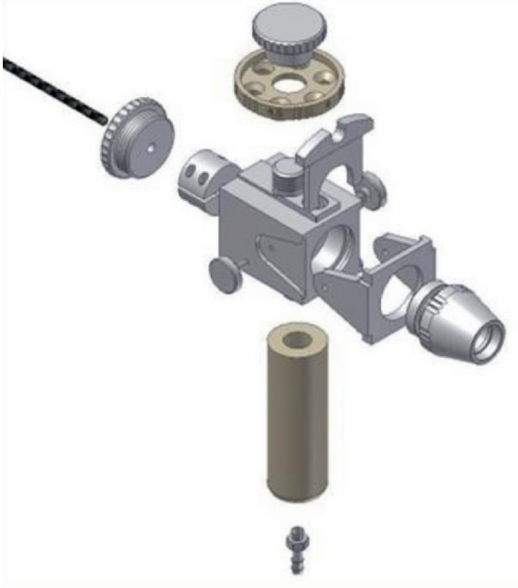
Figure 2: Test inhaler with the rotating disk having the three resistance orifices on top.
