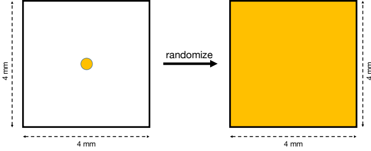
Figure 4.2: Randomization procedure of the LOR endpoints. The dot on the left shows the endpoint of each LOR before the randomization. The endpoint is randomly redistributed across the whole crystal surface.
