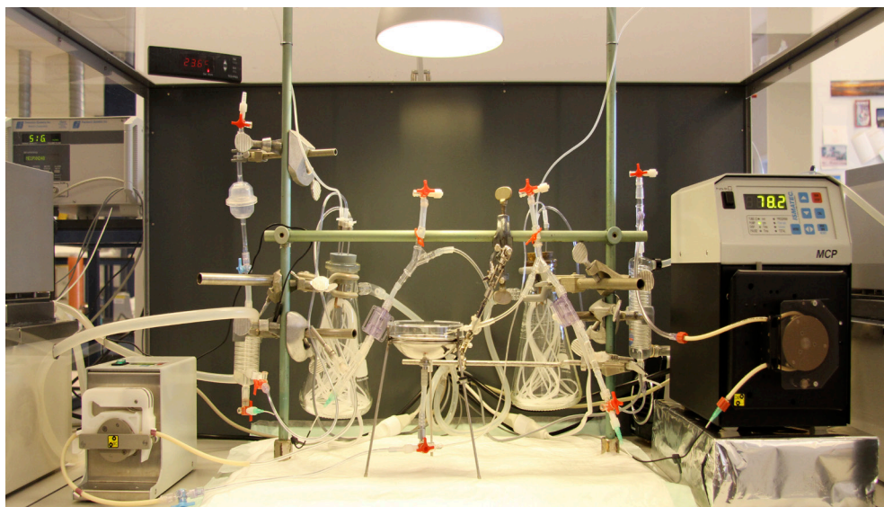
Figure 4. General overview of the rodent liver perfusion system. The system consists of a portal and arterial side and the whole system is situated inside a climate box. The laptop, flow meter and two water baths are located outside the box, and are connected into the enclosed system via an entry port.
